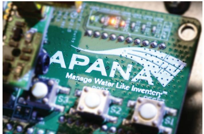
Apana. The solution was designed to track water usage every minute. Cellular technology was evaluated and found too power hungry to meet 1-minute requirements while maintaining a 10 year battery life. In addition, water meters are often located in difficult to reach areas for direct wiring and replacing batteries for frequently transmitting device was not an option.
