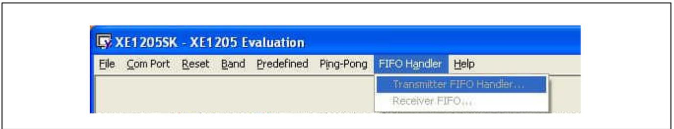
The Transmitter FIFO Handler function is only available if the XE1205SK is set in transmitter mode and if the Buffered mode is enabled. A message is displayed at the bottom right corner of the screen.
