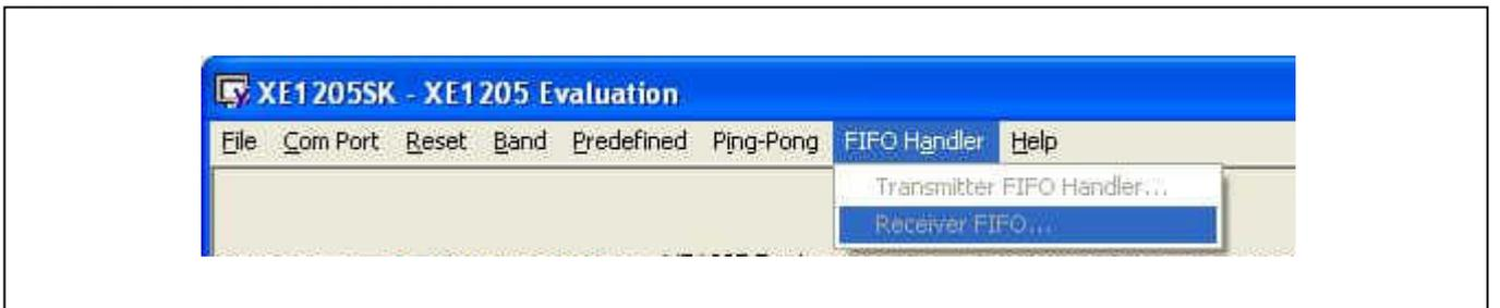
The Receiver FIFO is only enabled if the XE1205SK is set in receiver mode and if the Buffered mode is activated. A message is displayed at the bottom right corner of the screen.
