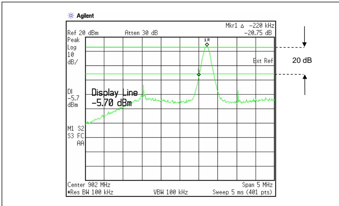
**Figure 5: Transient Band Edge Conducted Emissions Measurement**
