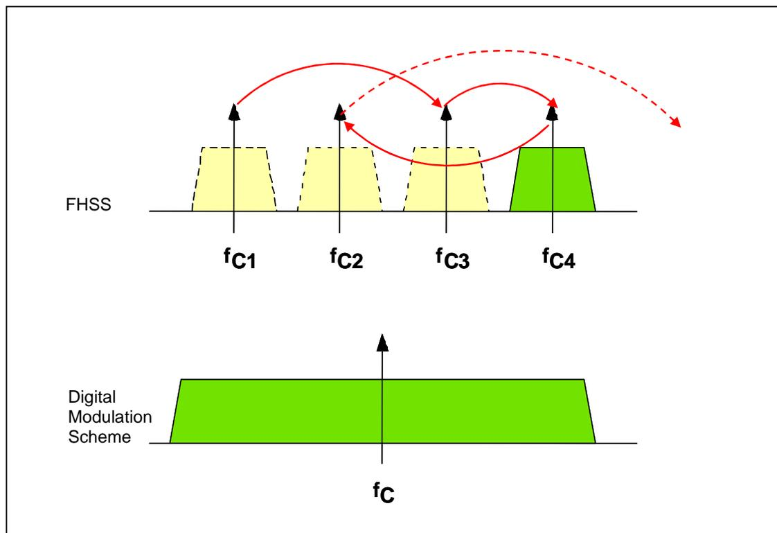
**Figure 1: FHSS and Digital Modulation Scheme Spectrums**
