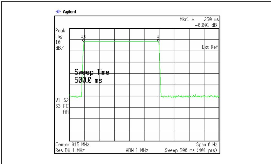
**Figure 4: Measurement of Hopping Channel Dwell Time**
