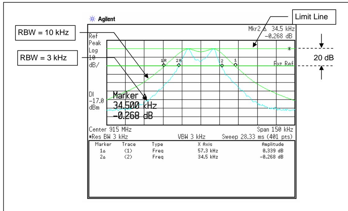
Figure 2: Measurement of 20 dB Bandwidth
