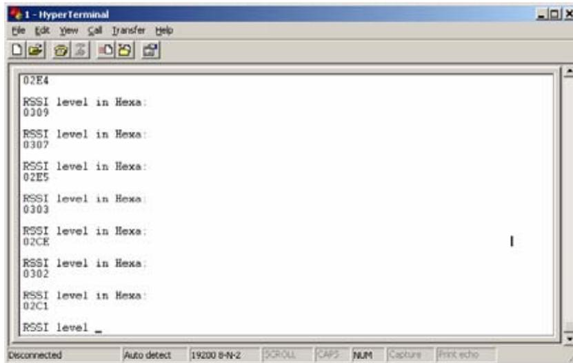
The return value is related to the 12 bit ADC. To get the received signal power in dBm, we should apply the formula 1 from section 2.
