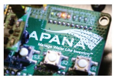
Apana. The solution was designed to track water usage every minute. Cellular technology was evaluated and found too power hungry to meet 1-minute requirements while maintaining a 10 year battery life. In addition, water meters are often located in difficult to reach areas for direct wiring and replacing batteries for frequently transmitting device was not an option.
