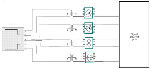
Figure 4 – RClamp 2502L Flow-through layout for Gigabit Ethernet Protection
