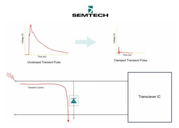
Figure 1 – TVS Diode Conceptual Operation
