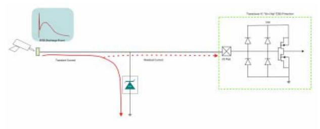
Figure 3 – TVS Diode on Dataline with representative "on-chip" ESD structure
