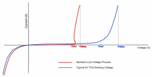
Figure 2 – IV Curve for Transient Circuit Protection Diodes
