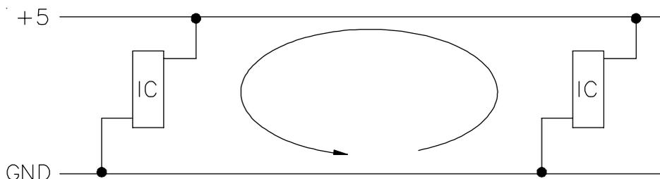
**Figure 1 - Power and Ground PCB Loop**
