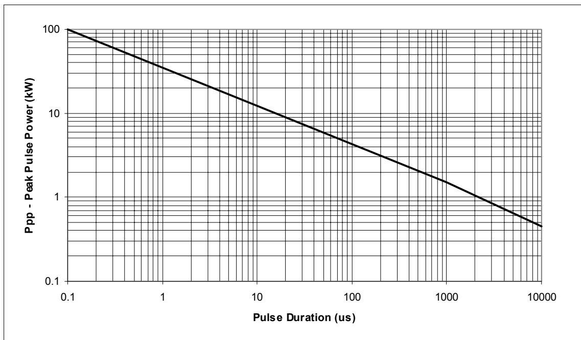
Figure 1 - Peak Pulse Power vs. Pulse Duration for a 1500W TVS Diode
