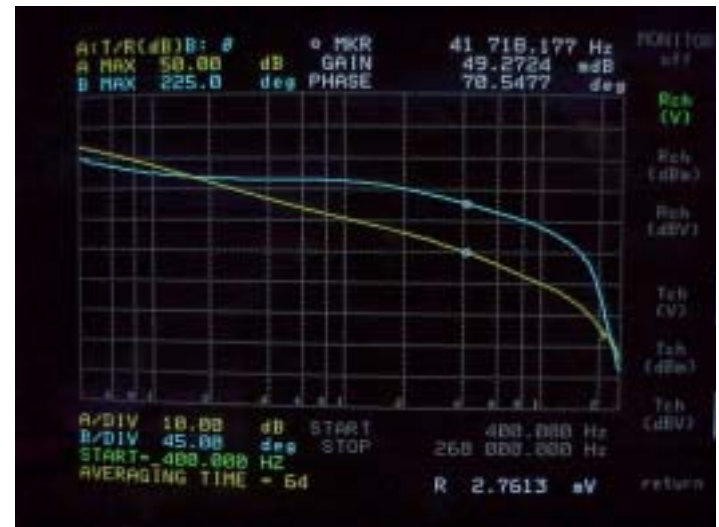
Fig. 6 - Measured loop gain Bode plots.
